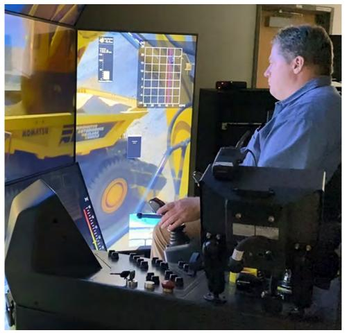
Komatsu's real time teleoperated excavator in action.
