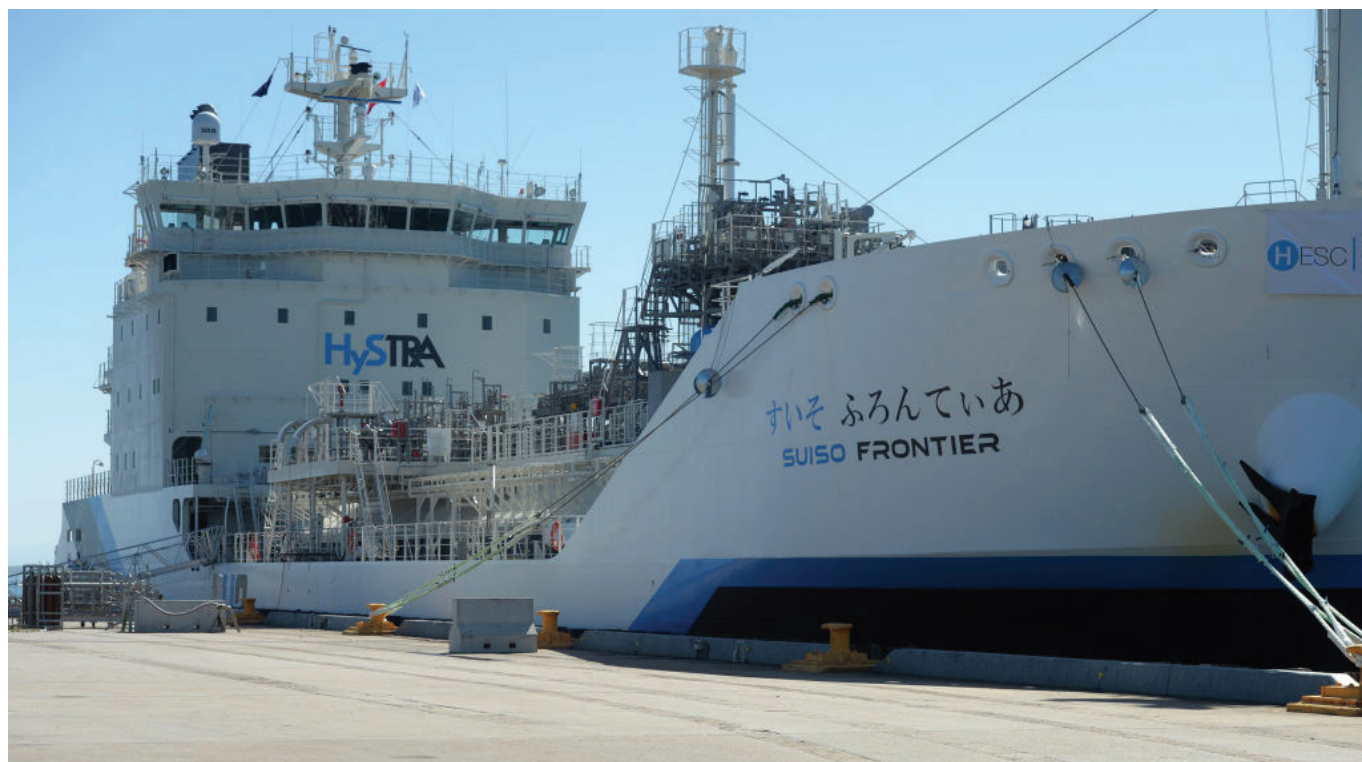
The Suiso Frontier, world's first vessel capable of shipping liquid hydrogen over intercontinental distances.
